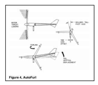
The thrust force acts through the centerline of the rotor, which is offset from the centerline of the tower pivot axis (yaw axis). Therefore, the thrust force on the rotor is always trying to push the rotor over to the side, away from the wind.
