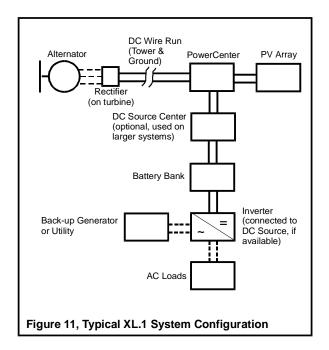
The PowerCenter has a limited current carrying capacity so we recommend that you use a DC Source Center whenever you have multiple XL.1 wind turbines. DC Source Centers are available from Bergey Windpower.
