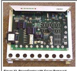
Figure 13, PowerCenter with Cover Removed
