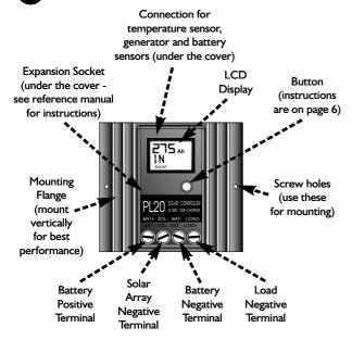
Screw wires into these terminals *tightly* as described on page 4.
